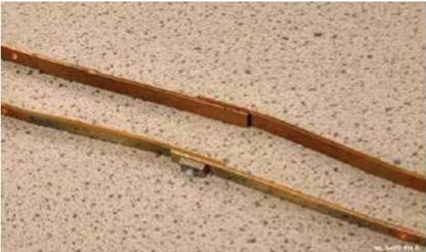
Fig. 6. Lap and bolted lap joints after short-circuit test.
