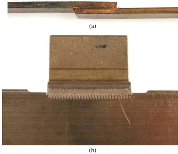
Fig. 3. Joints. (a) Lap joint. (b) Edge joint.
